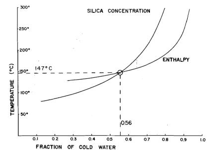
Fig. 8 Graph illustrating a mixing model calculation of a silica predicted temperature for the undiluted reservoir at Cabarton Hot Springs at the south end of Cascade Reservoir. The predicted reservoir temperature is 147°C with 56% cold-water dilution for the spring.
