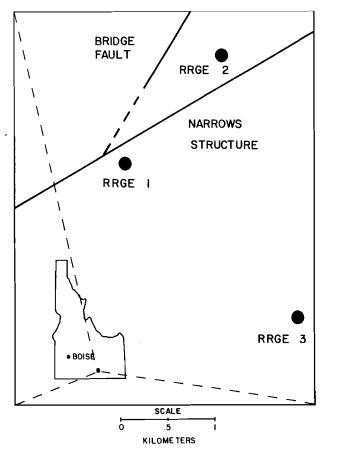
Fig. 9. Schematic map of the Bridge fault, the Narrows structure, and RRGE 1, 2, and 3. The Bridge fault is along the eastern flank of the Jim Sage Mountains, and the Narrows structure separates the Jim Sage Mountains from the Raft River Mountains (Fig. 10).
