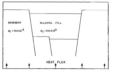
Fig. 12. Schematic diagram of the proposed geological model for the Boise, Cascade, and Raft River geothermal systems. Thermal conductivities ( $\sigma$ ) of 3.0 x 10<sup>-3</sup> and 7.0 x 10<sup>-3</sup> cal/cm s <sup>o</sup>C were used for the sediments and basement rock, respectively, to calculate the temperatures at the base of the sedimentary section.
